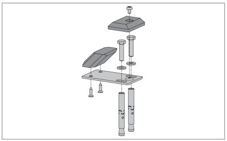
Install the floor guide for the PAMH60 door wing by complying with the measurements on page 8 [VALORHH], or on page 10 [VALORHS].
