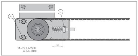
Loosen the screws [A], unscrew screw [B] until the spring compresses to 22 mm (if the length of the automation is less than 2600 mm) or 20 mm (if the length of the automation is more than 2600 mm).
