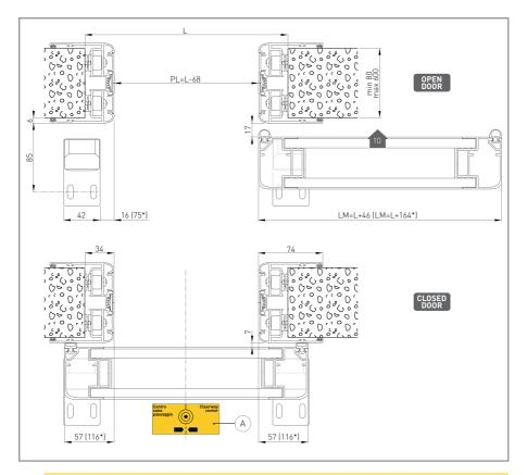
WARNING: fasten the automation to the wall so that the label [A] on the box coincides with the centre of the doorway.
